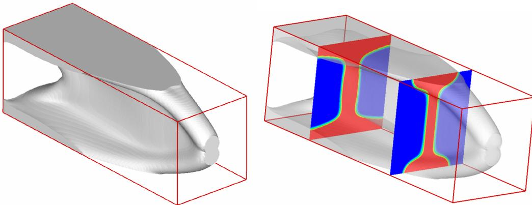
**FIGURE 3.** A cantilever beam design solved using the preconditioned, recycling MINRES solver and the CAMD approach; mesh size:  $210 \times 70 \times 70$  B8/B8 elements; total number of unknowns: approximately 1.6 million. Left: final design of a homogeneous material. Right: Two cross-sections from the final design.
